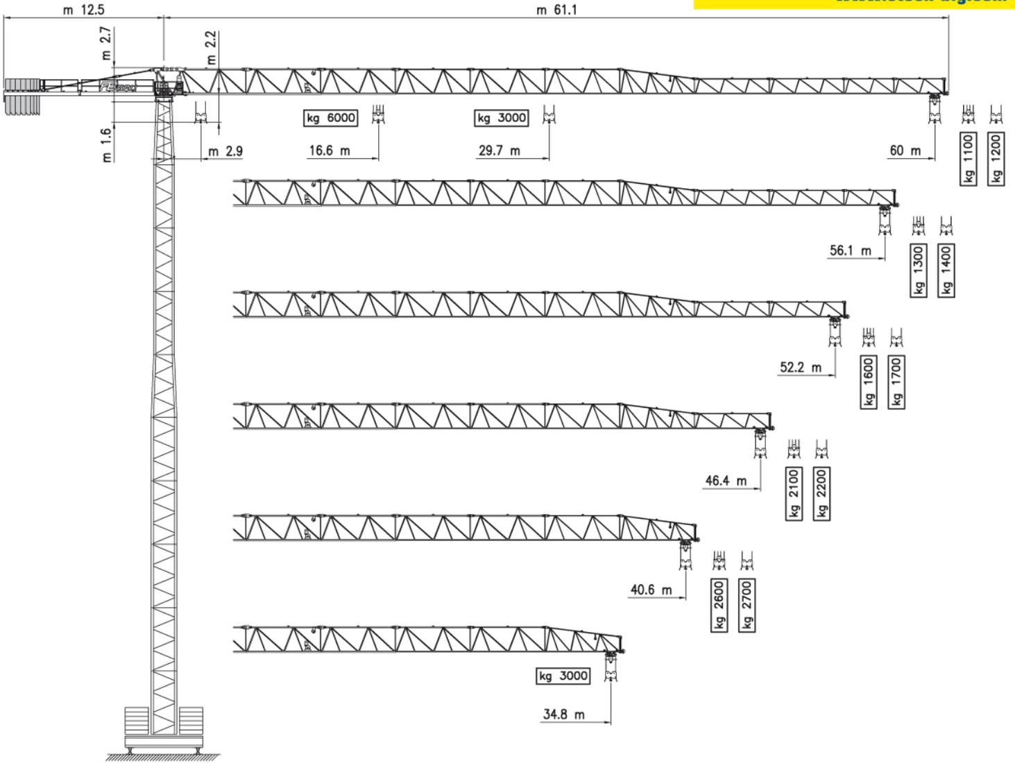
**CURVE DI CARICO** CURVAS DE CARGAS — LOAD DIAGRAMS
