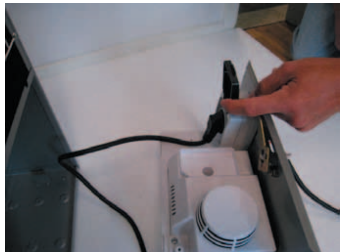
Connect the power supply cable to the socket in the pump unit.
