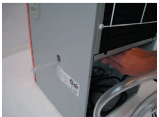
Insert the hose through the hole on the side of the dehumidifier.
