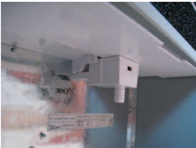
Mount the adaptor in the slot underneath the run off sheet.
